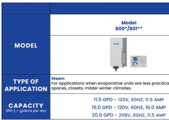
\*Model 800LC available for low conductive water 75-300uS/cm and 120VAC applications. \*\*801 & 866 Modulating Steam Humidifier – For precise RH control. Controls are sold separatel
